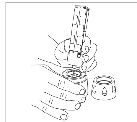
Drawing 8 - Correct insertion of the battery casing
